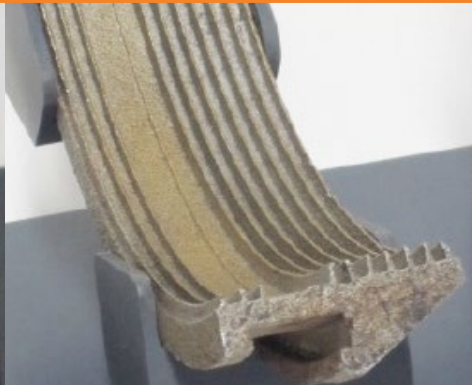
Chemical Corrosion on Aluminum Seal
