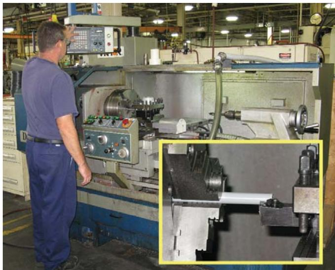
*This Quadrant gray Radel® PPSU 1000 is being turned during the manufacture of a medical instrument handle. Quadrant's expanded line of Radel PPSU 1000 colors includes more sizes of rod and sheet and is used for many life science applications.*
